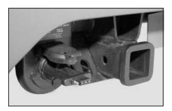
Connect the adapter with the tab pointing up. Then flip cap on the vehicle's seven-wire harness will lock onto the tab and help hold the adapter in place. Plug the four-way round pin connector onto the adapter.
